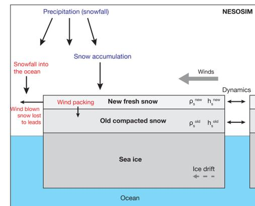
Figure 5: Schematic of the two-layer Eulerian snow budget model. The red (blue) text indicates processes that result in a loss (gain) of snow depth.
