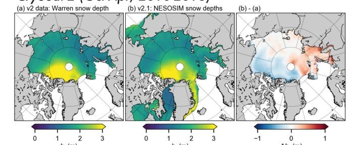
Figure 8: Comparison of the winter (October-April) 2010-2016 Arctic CryoSat-2 sea ice thickness including (left) new waveform tracker and the Warren snow depth climatology and (middle) using the updated NESOSIM daily snow depth/density data.
